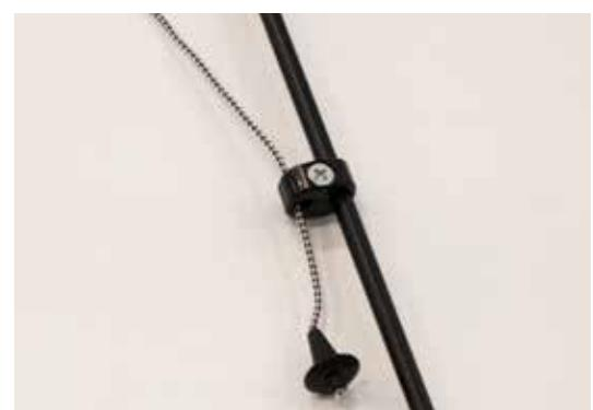
Guide-rod-stopper with aluminium base for glass gluing.
